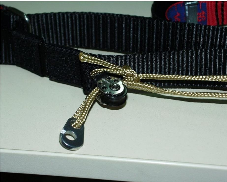
The line length is universal – fits to all our Dudek's paragliders. The pilot should knot the line such a way, that hook “touches” the upper pulley on the riser while the riser is fully extended.
